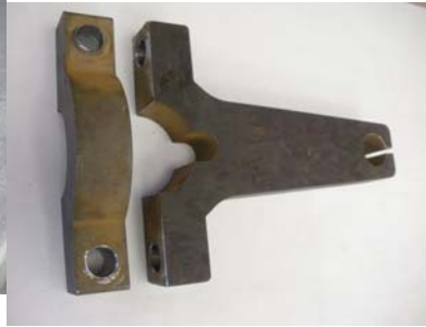
Our machining centers drill and tap the parts
