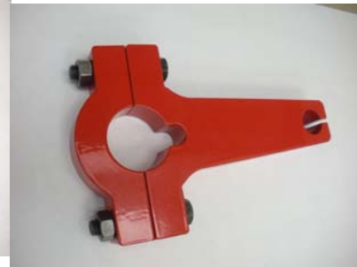
Part is powder-coated, and assembled for shipment to client
